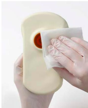
**Figure 17. Cleaning the Bottom of the SEM Scanner**
