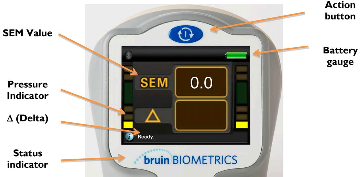
**Figure 4. SEM Scanner Display (V3.60)**
