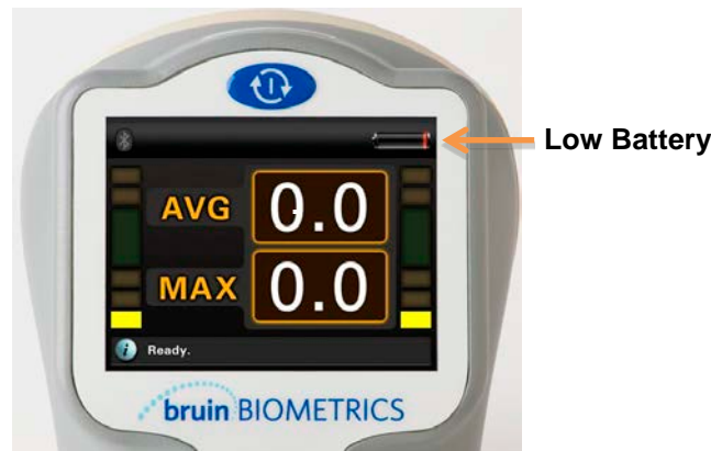
Figure 6. The battery gauge is in the upper right corner of the SEM Scanner Display
