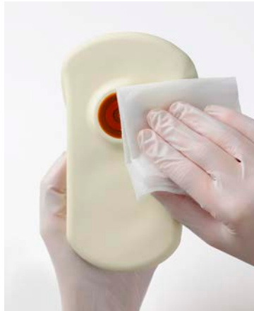
Figure 14. Cleaning the Bottom of the SEM Scanner
